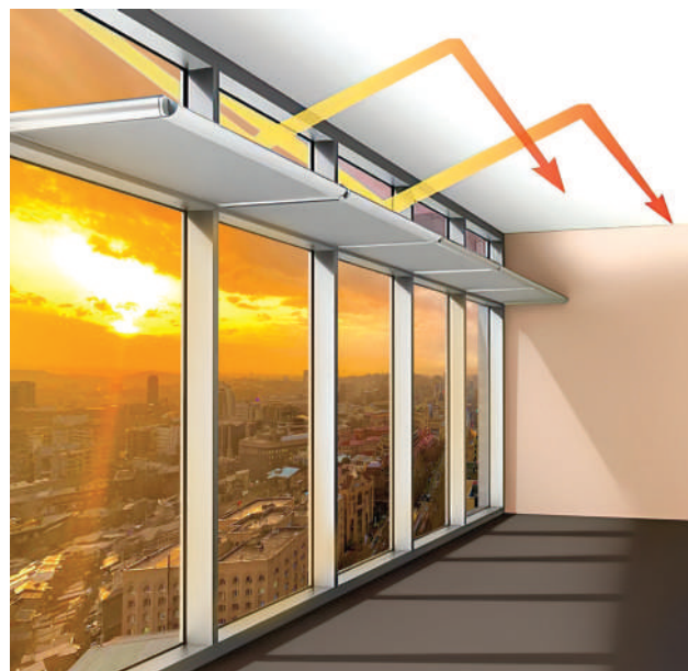
Figure 30. Example of light shelves reflecting the light deeper into the room
