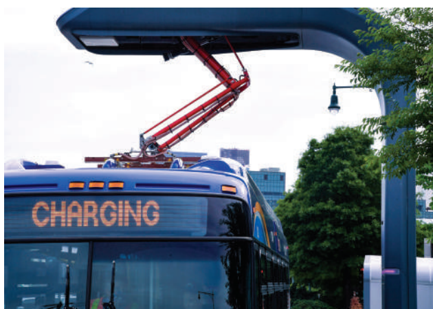
Figure 14. Example of Electric Bus Charging Station
