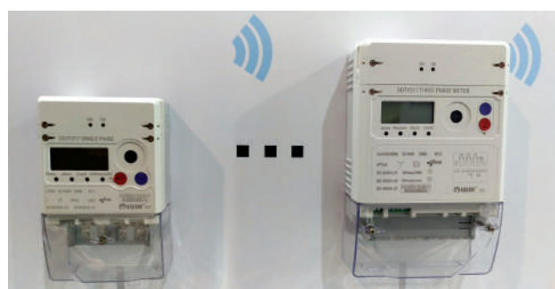
Figure 50. Example of smart meters
